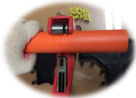
Cut the sheath by round cutter
