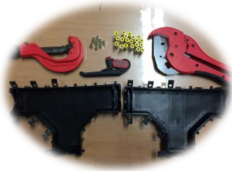
Prepare T branch closure, tools, connectors, etc.
