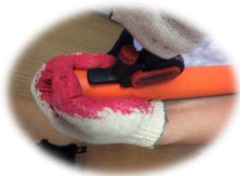
Remove the sheath by using splitter.
